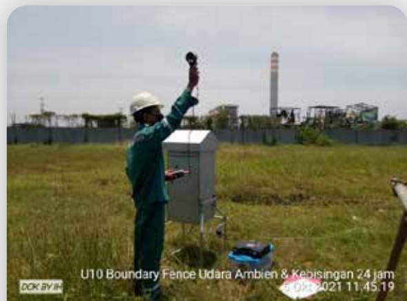
Monitoring kualitas udara Ambient dan Kebisingan di area proyek Air Ambient Quality and Noise monitoring at Project area
